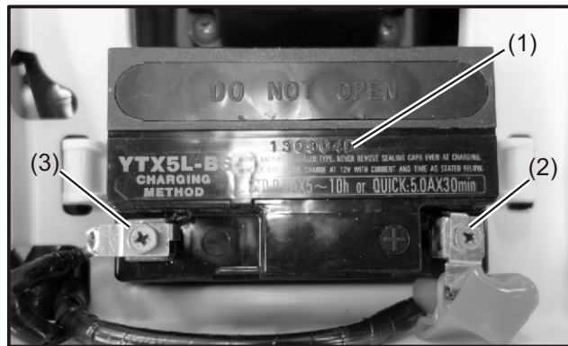
(1) Battery (2) Positive (+) terminal lead (3) Negative (-) terminal lead
