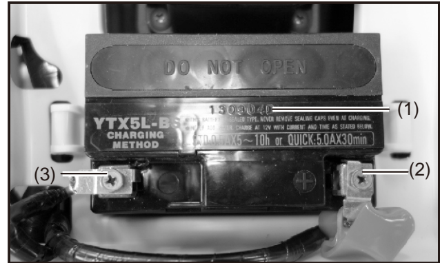
(1) Battery (2) Positive (+) terminal lead (3) Negative (-) terminal lead
